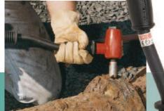
Reduce dust and hazardous particles in work area with optional vacuum shroud for Heavy-Duty Hand-Held Scabblers (below).
