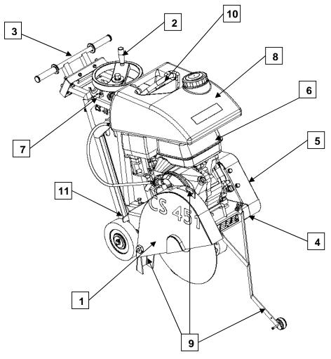
Made of jig welded open profile steel, the **CS 451** is stable but at the same time, easily transportable.
