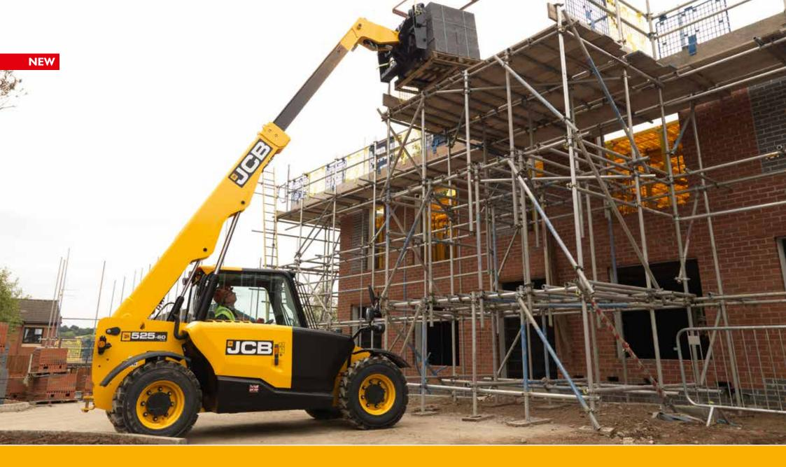
LOADALL | 525-60 HI VIZ Gross power: 55kW/74hp Lift capacity: 2,500 kg Lift height: 6.0m
