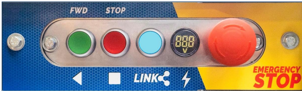
Start and mid conveyors in the run have illuminated LINK button
