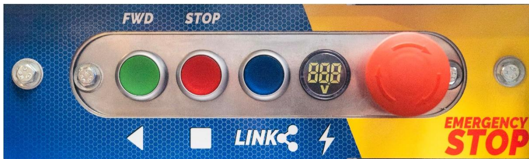
End conveyor of ANY run to have the LINK button out and not illuminated
