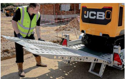
The Rhino comes with three different ramp options: full width, individual and double angle. Choose between 1400mm and 1700mm loading ramps to suit your requirements.
