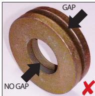
DO NOT FIT DISC SPRINGS LIKE THIS
