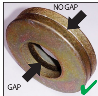
FIT DISC SPRINGS LIKE THIS
