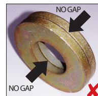
DO NOT FIT DISC SPRINGS LIKE THIS
