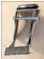
Side impact and foot pedal distortion as a result of a significant side impact.
