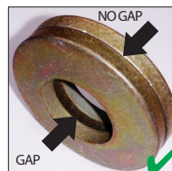
FIT DISC SPRINGS LIKE THIS
