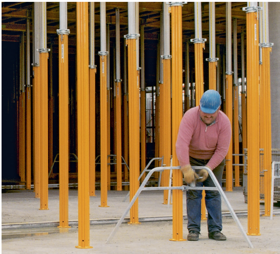
The Universal Tripod is used as an erection aid. Horizontal loads have to be transferred through the formwork to the structure.
